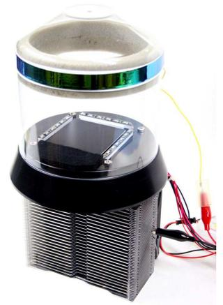
With the new EX-type, observation area is enlarged to 60mm × 60mm. Large cylindrical chamber enable multi-people observation, and very high efficiency enable observation of natural-radiation .
