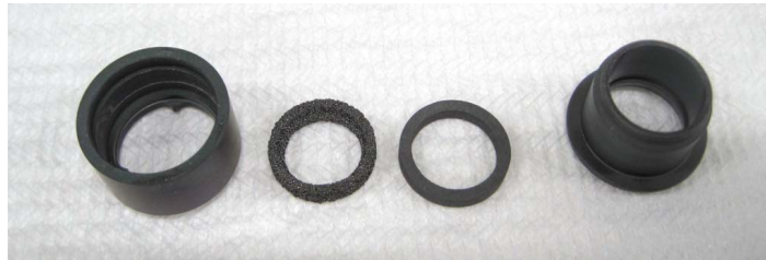
D3 Specimen holder manufactured by Mo-TEM alloy.
