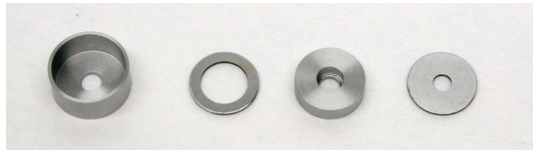
D3 Specimen holder manufactured by Mo-TEM alloy.
