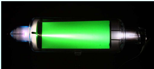
A Crookes tube operated by 5kV (Horizon Co. VT-7010)
