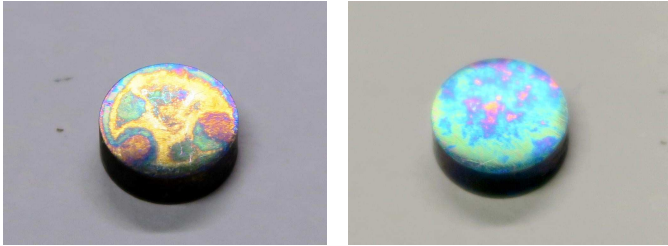
K-doped W-3%Re and Pure W after the measurements up to 500°C in vacuum via RP using LFA-457.
