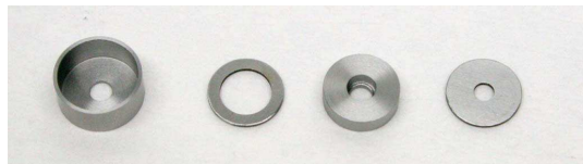
D3 Specimen holder manufactured by Mo-TEM alloy.
