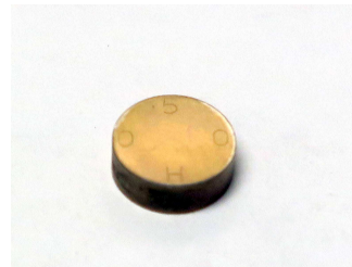
Ar leak from a valve inside of LFA-467HT cabinet gives a slight oxidation after a measurement up to 800°C on Pure W.
