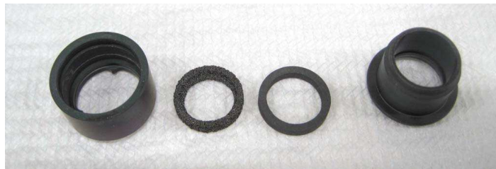
D3 Specimen holder manufactured by Mo-TEM alloy.
