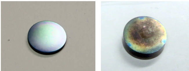
Pure W (ITER-G) and tungsten side of W/SiC after a measurement up to 500°C and 800°C with Ar flow using LFA-457.
