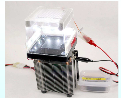
Main unit of standard type (SD) Peltier-cooling cloud chamber.
