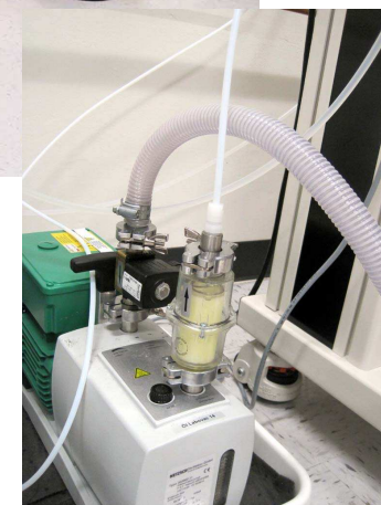
RP exhaust → Evacuation Port
