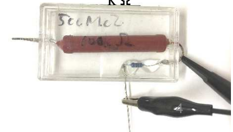
Voltage divider 500 MΩ + 100 kΩ
